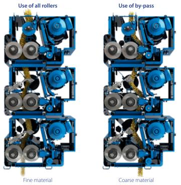
The coarse material can be transported through 1,2 or 3 pairs of rollers, each pair with different riffles. This is completely flexible so the fineness of structurizing can be controlled completely.
